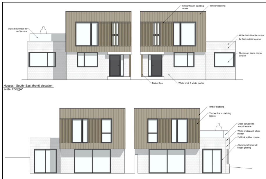
Fig.6: Front and rear elevations of proposed houses
